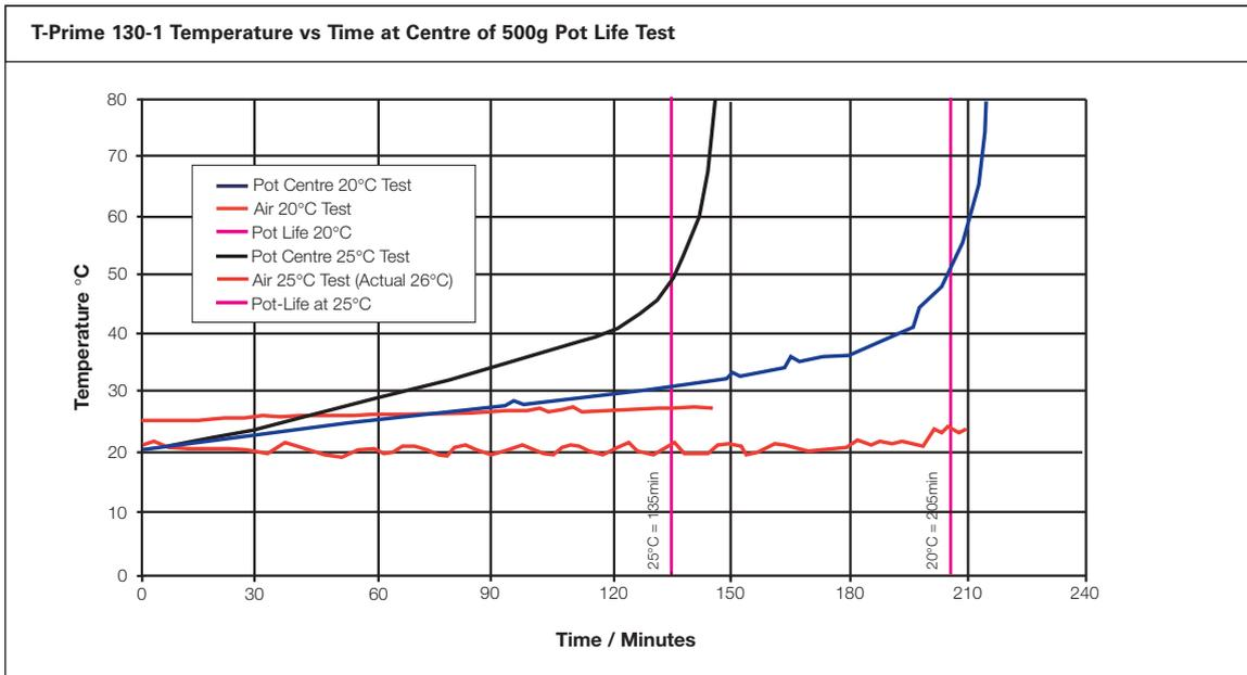
Large volumes of T-Prime 130-1 left in bulk > 50mm deep can exotherm strongly and the excess will need to be dispensed into a shallower vessel. Ideally this should be less than 30mm deep or the pot placed into water to cool.
